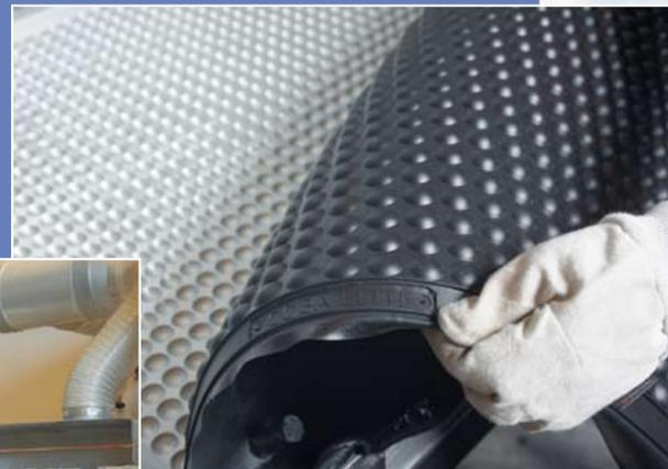
*PUR in two widely different ways! Noise-absorbing motor suspension made of compression-moulded PUR foam for vacuum cleaners, and a workplace mat made of flex integral, being removed from their moulds. PUR features challenging versatility.*
